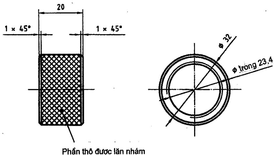
**Hình C.4 – Khớp nối**
